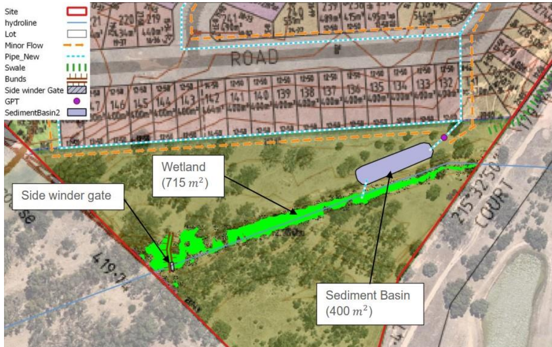
Figure 2-5 Proposed location and extent of the wetland and sedimentation basin proposed for Option 2 of the stormwater management structures for the proposed residential development (Afflux Consulting 2023).
