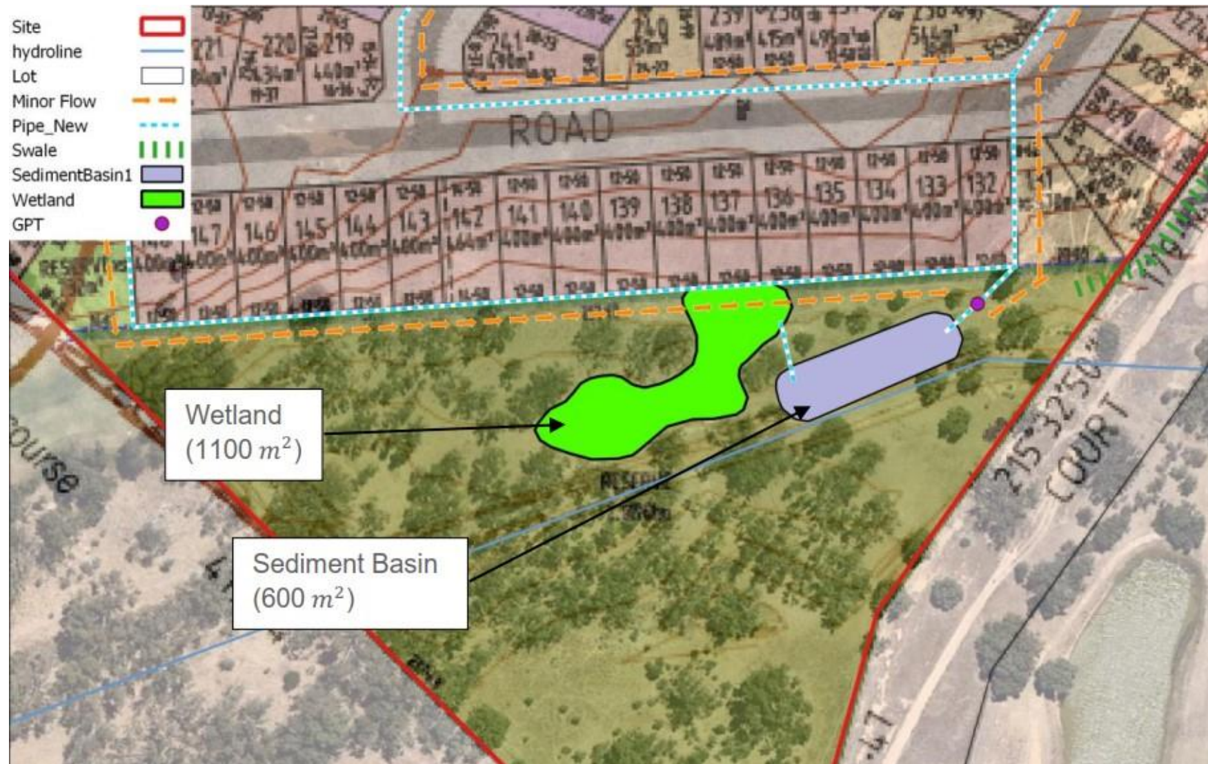
Figure 2-4 Proposed location and extent of the wetland and sedimentation basin proposed for Option 1 of the stormwater management structures for the proposed residential development (Afflux Consulting 2023).
